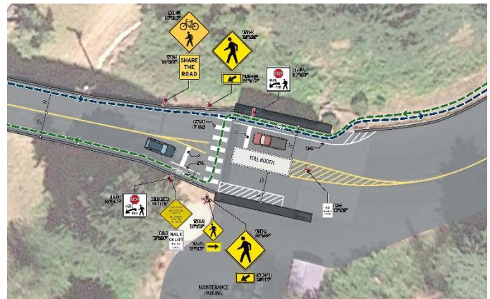
Proposed Safety Enhancements around the toll booth to provide better access for pedestrians.
